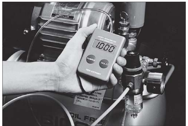
▲ Measurement of source pressure from a compressor.
