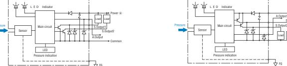
Change in the pressure indication, switch operating points and analog output.
