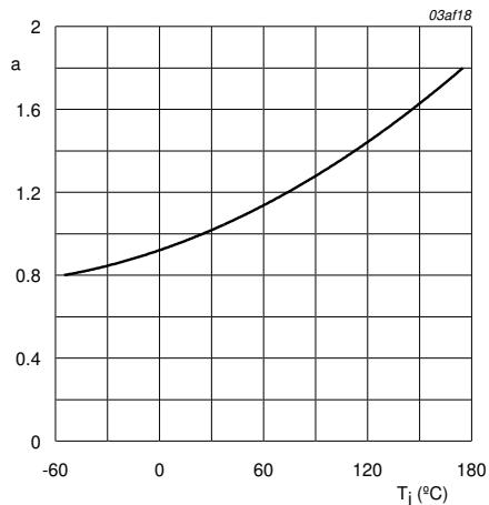
$$a = \frac{R_{DSon}}{R_{DSon}(25^\circ\text{C})}$$
