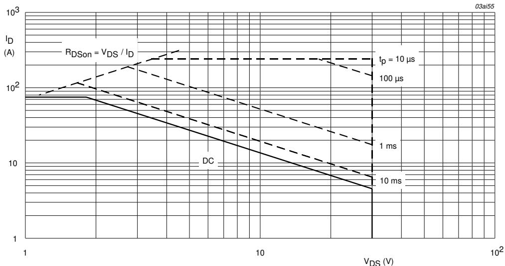
T<sub>mb</sub> = 25 °C; I<sub>DM</sub> is single pulse; V<sub>GS</sub> = 10V.
