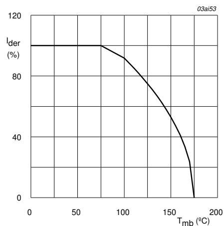
$$I_{der} = \frac{I_D}{I_{D(25^{\circ}\text{C})}} \times 100\%$$
