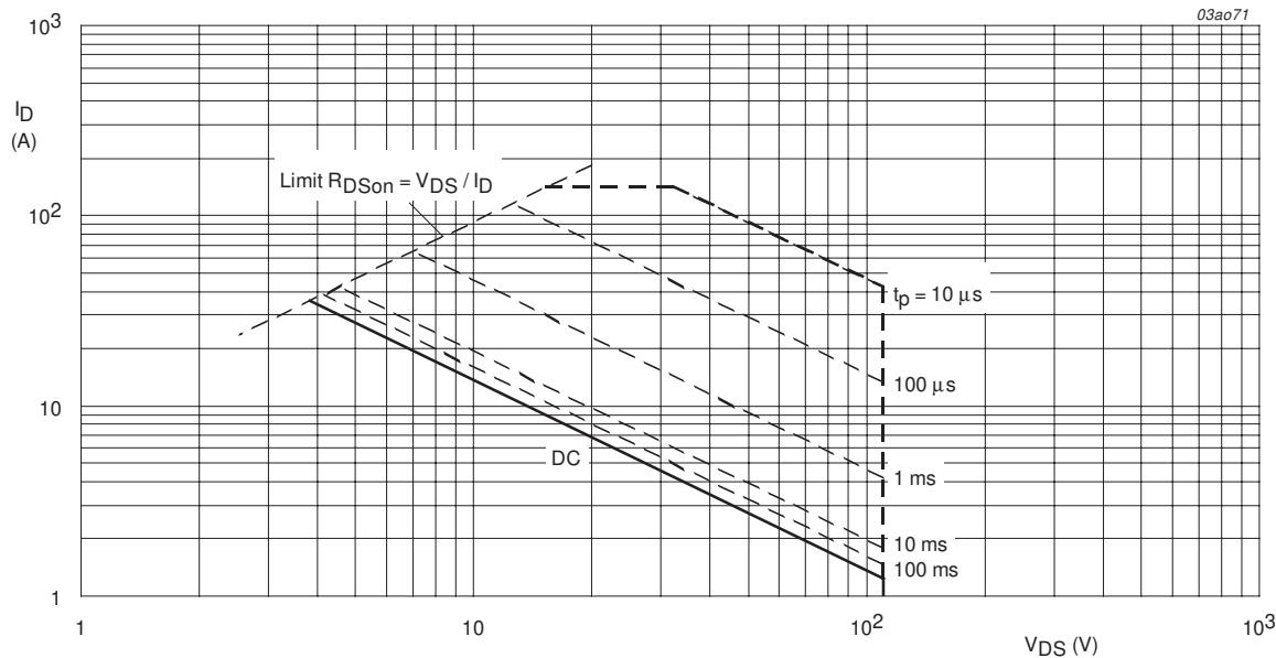
$T_{mb} = 25^{\circ}C$ ;  $I_{DM}$  is single pulse;  $V_{GS} = 10$  V.
