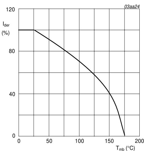
$$I_{der} = \frac{I_D}{I_{D(25^{\circ}C)}} \times 100\%$$
