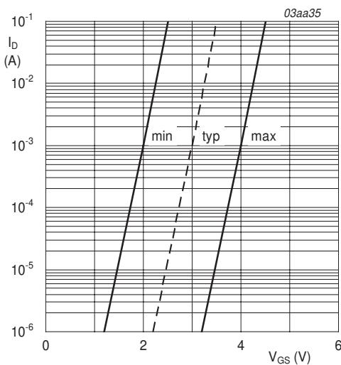
$T_j = 25 \text{ }^\circ\text{C}; V_{DS} = 5 \text{ V}$
