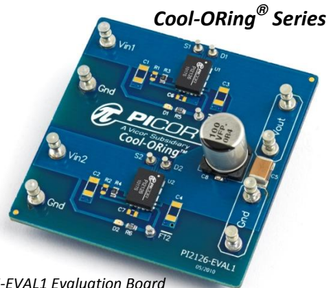
PI2126-EVAL1 Evaluation Board featuring the Cool-ORing PI2126 Full-Function Active ORing Solution.
