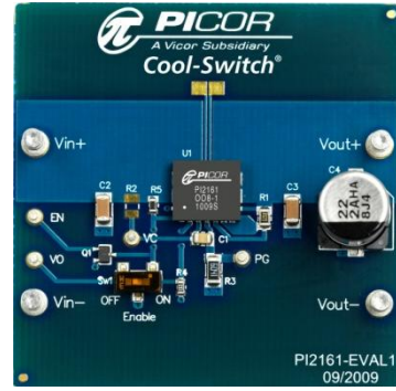
Figure 1: PI2161-EVAL1 Evaluation Board (1.8" x 1.8")
