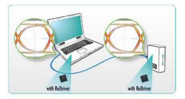
Redrivers with emphasis and equalization signal conditioning technology ensure the integrity of high-frequency PCIe 2.0 signals by opening closed signal eyes to recover data and meet strict compliance testing requirements. Increased signal margin also supports longer drive lengths over even low-quality cables.
