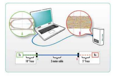
PCIe 2.0 signals must not only run reliably over varying lengths of cable but also across multiple connectors and traces between the transmitter and receiver.
