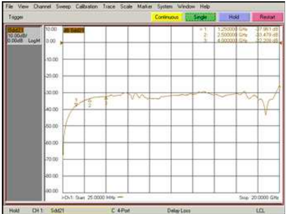
Fig 4. Differential Crosstalk – Super Speed
