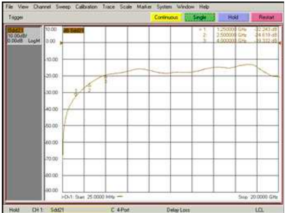
Fig 5. Differential Off Isolation – Super Speed
