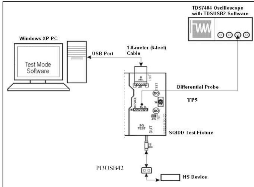
**USB2.0 High-speed (480Mbps) Signal Integrity Test Setup**
