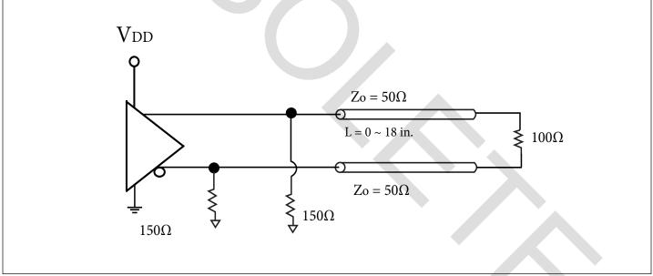
Figure 5. LVPECL output termination
