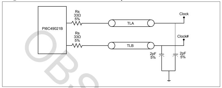
Figure 4. Configuration Test Load Board Termination
