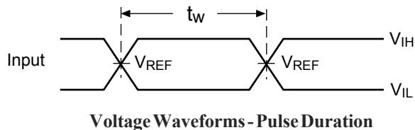
**Voltage Waveforms - Pulse Duration**
