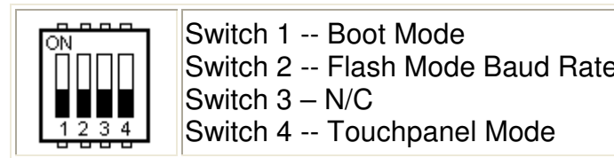
Figure 5. DIP Switch Settings
