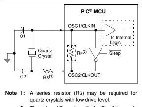
2: The value of RF varies with the Oscillator mode selected (typically between 2 M $\Omega$  to 10 M $\Omega$ ).
