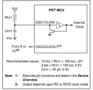
In RCIO mode, the RC circuit is connected to OSC1. OSC2 becomes an additional general purpose I/O pin.
