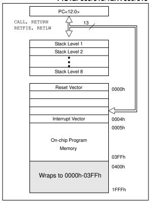
FIGURE 2-2: PROGRAM MEMORY MAP AND STACK FOR THE PIC12F617
