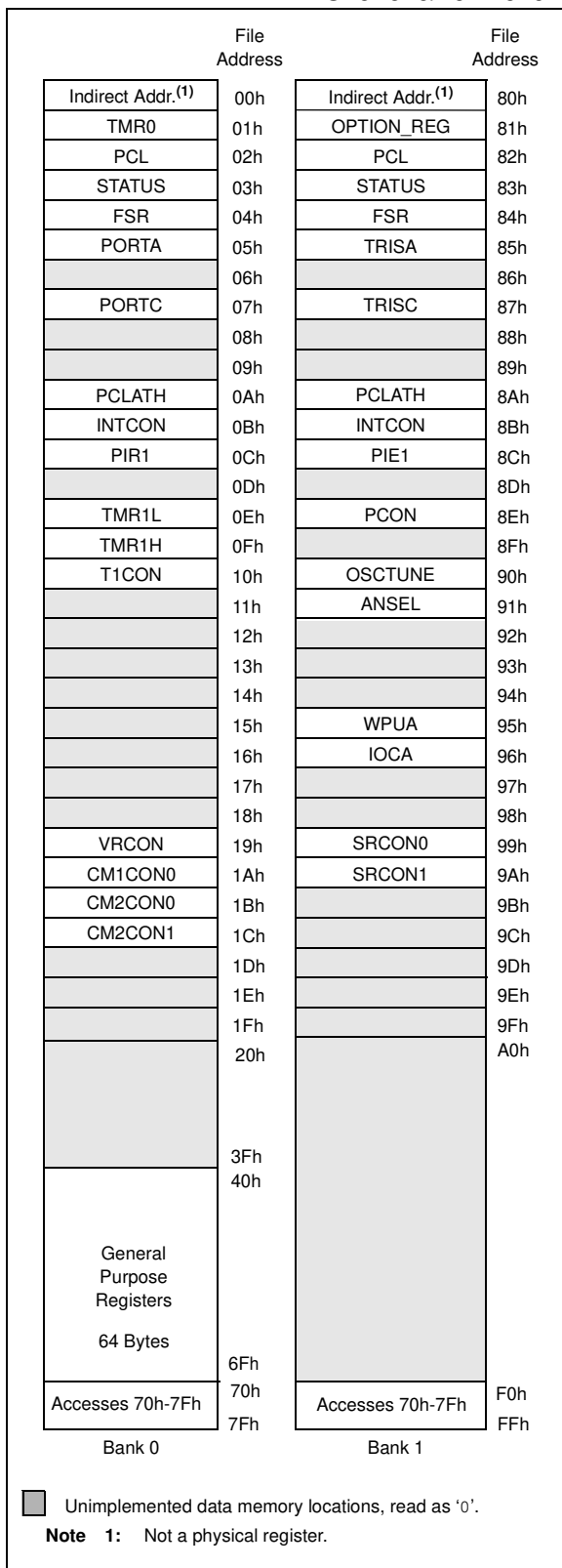
FIGURE 2-3: DATA MEMORY MAP OF THE PIC16F610/16HV610
