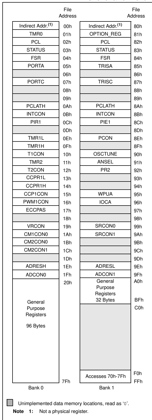
FIGURE 2-4: DATA MEMORY MAP OF THE PIC16F616/16HV616
