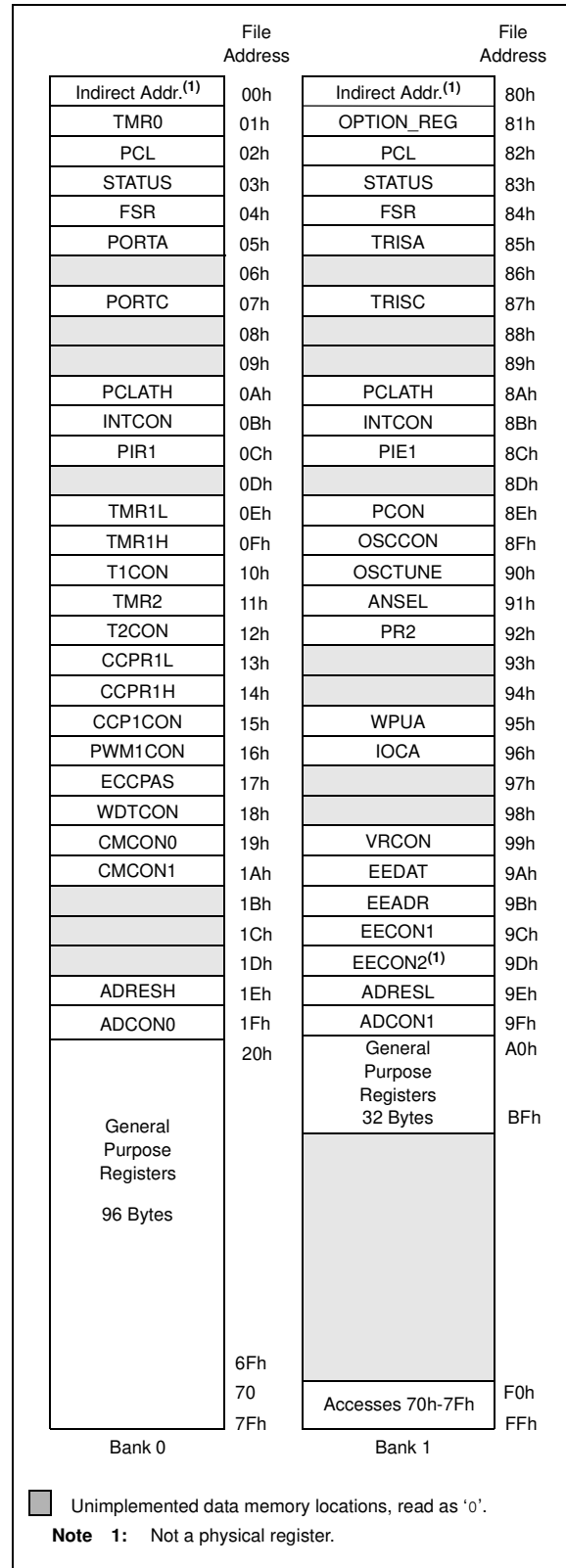
FIGURE 2-2: DATA MEMORY MAP OF THE PIC16F684
