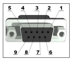
**TXD** is an output. It is the "Transmit Data" signal which is the asynchronous serial data output (RS232) for the shift register on the UART controller.
