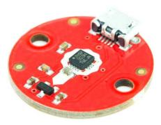
The Motion module can detect motion in three axes - X, Y, and Z as well as being able to detect compass heading. Ideal for building into robots, or as a tilt-sensitive controller for games.
