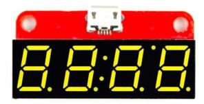
The Number module is a seven-segment display, with four digits, four decimal points, and a colon between the two pairs of digits. It's ideal for using as a readout of sensor values, as a clock, or a countdown timer.
