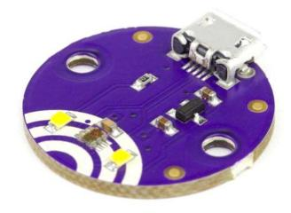
The Colour module detects RGB colour, as well as ambient light level. It also has two bright white LEDs to illuminate objects whose colour is being detected.
