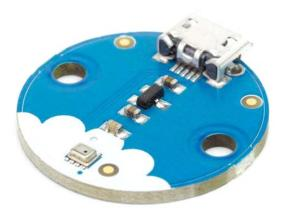
The Weather module reads temperature and pressure. It's ideal for setting up a mini weather station to monitor conditions in your house or garage.
