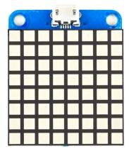
The Matrix module is an 8x8 white LED matrix. It's perfect for scrolling text on, displaying simple animations like smiley faces, or using as a tiny marble maze.
