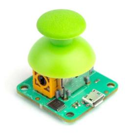
The Joystick module is an analog joystick with a click button. It's ideal for using as a game controller, or to control a robot.
