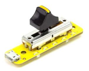
The Slider module is a slide potentiometer which has five bright white LEDs that illuminate as the slider is moved. It's perfect for using as a synth controller or for controlling the speed of your robot.
