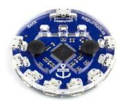
The Flotilla Dock is the heart of the Flotilla system. It talks, through serial USB, to all of the Flotilla modules connected to its eight ports. Connect it to your Raspberry Pi with a good quality USB A to micro B cable, and then connect your Flotilla modules to the eight ports with Flotilla cables.
