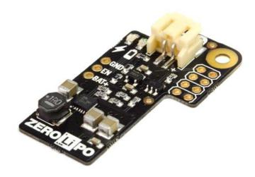
The tiny little LiPo/LiIon power supply shim for all versions of the Raspberry Pi!
