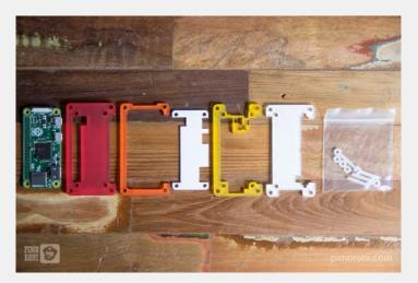
All you'll need is a Pi Zero and Pibow Zero. A screwdriver is optional, as you should be able to tighten the nuts by hand.
