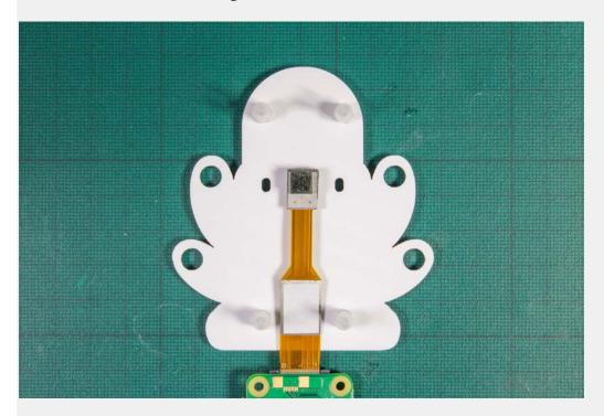
Now, fold the Pi Zero W over carefully, making sure that the camera lens stays located in the hole in the OctoCam mount. Slip the Pi Zero W down onto the bolts and use the remaining four nuts to secure it.
