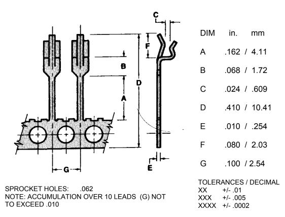
MATERIAL: Pre-Tin Plated Half Hard Phosphor Bronze .010 In. Thick RoHS Compliant PACKAGE: Rolls of 1000 pieces with paper interleaf.
