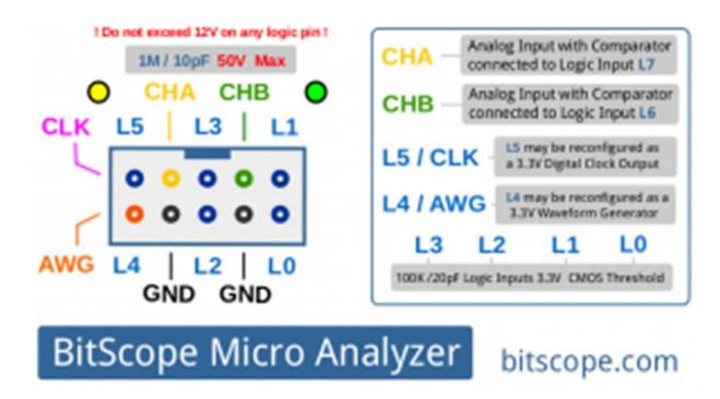
It's conveniently arranged so the two ground pins can pair with the analog inputs, waveform and clock generator outputs or logic inputs L0, L2 and L4. Like all BitScopes this model can capture 8 logic/timing channels but in this case logic channels L6 and L7 are derived from the analog channel comparators. This is a very powerful feature because it means the voltage ranges and switching levels for those two channels can be adjusted to suit almost any logic family, even inverted ones!
