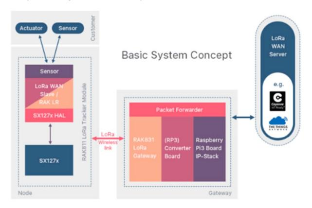
The RAK831 Pilot Gateway is the central hardware solution for all LoRa based radio communication. It receives and transmits radio messages. Processing of the radio messages as well as the protocol related tasks is done by the embedded host system (Raspberry Pi). Received and processed radio messages are being sent to a LoRaWAN server. The concrete segmentation of the protocol related tasks is outside the scope of this document.
