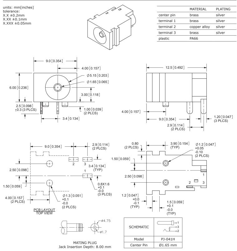
1. All specifications measured at 10~35°C, humidity at 45~85%, under standard atmospheric pressure, unless otherwise noted. Note: ..... ..... CUI Inc | MODEL: PJ- 041H | DESCRIPTION: DC POWER JACK
