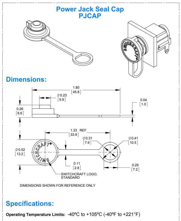
Weathertight Ratings: IP66, IP67, IP68 per IEC60529, NEMA 250 (6P)
