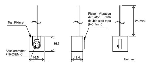
Total weight of Fixture and Accelerometer : 20g
