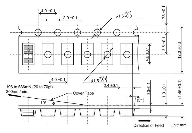
Figure.3 Dimension of Plastic Tape
