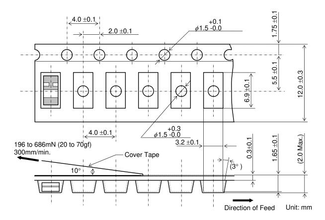
Figure.3 Dimension of Plastic Tape
