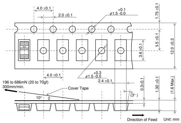
Figure.3 Dimension of Plastic Tape
