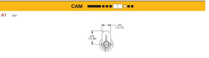
NOTE: Cam not assembled to switch. Other cam lengths and styles available, consult Customer Service Center.
