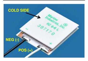
Thermoelectric coolers (TECs) are mounted using one of three methods: adhesive bonding, compression using thermal grease or solder.
