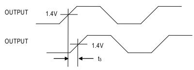
**Input-Output Propagation Delay**
