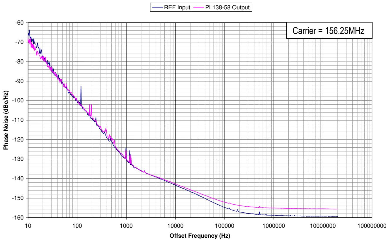
When a buffer is used to pass a signal then the buffer will add a little bit of its own noise. The phase noise on the output of the buffer will be a little bit more than the phase noise in the input signal. To quantify the noise addition in the buffer we compare the Phase Jitter numbers from the input and the output. The difference is called "Additive Phase Jitter". The formula for the Additive Phase Jitter is as follows:
