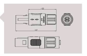
A3 Straight plug with cable collet and nut for bend relief
