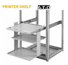
The Printer Shelf is used for supporting a continuous feed printer. The shelf mounts directly to a PROLINE™ frame. Paper shelves are vertically adjustable. The entire unit slides out 17 in. from the enclosure, allowing easy accessibility. Fits 600- or 800-mm wide frames that are 600-mm or more deep.
