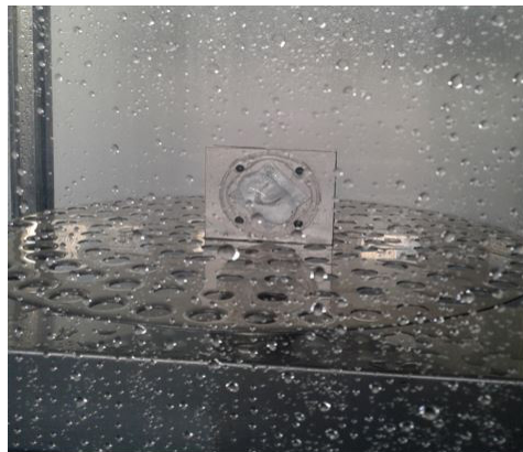
Testing under water jet
