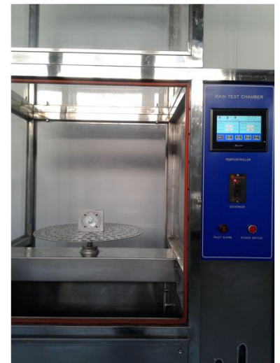
Testing under water jet
