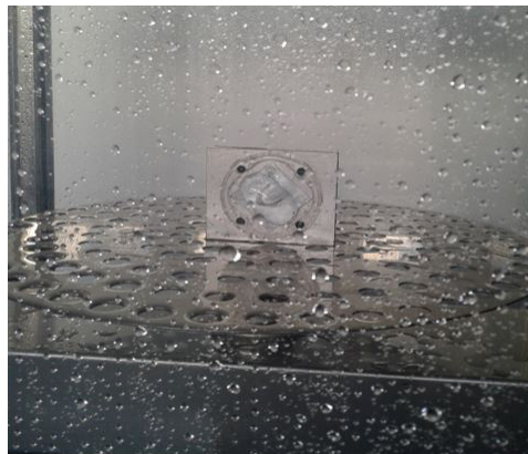
Testing under water jet
