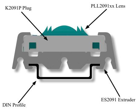
PLL2091xx Lens series is compatible with DIN Profile Standards:
