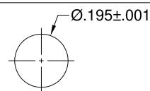
Recommended Mounting Holes Panel Thickness: 0.047"-0.093"
