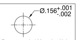
Recommended Mounting Holes Panel Thickness: 0.047"-0.093"
