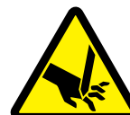
W3158 Cut or Sever Hazard
