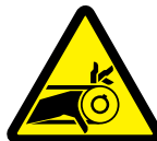
W3154 Belt Drive Entanglement Hazard
