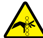
W3153 Pinch Point Hazard
