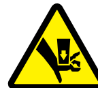
W3152 Crush Hazard
